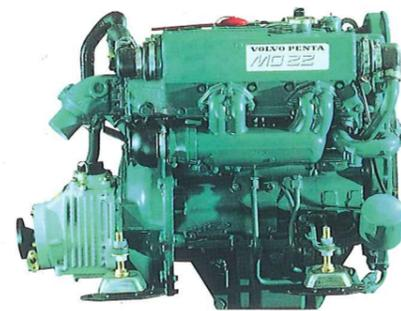
Volvo Penta MD22, 4 cylinder direct injection 4-stroke marine diesel with fresh water cooling. Power output at propeller, 42 kW (57 h.p. at 4,000 r.p.m.). Mechanical reverse gear MS2 B with single lever control, reduction ratio 2.4:1. Propeller shaft of 35 mm acid resistant stainless steel. Stern tube water lubricated rubber bearings. 3-bladed fixed propeller in bronze, pitch 13", diameter 17" left handed.
