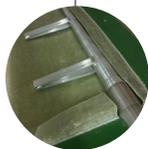
The balanced spade-rudder, with self aligning bearings, is made in glass fibre reinforced vinylester, with a divinacell core.
