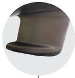
The lead keel is moulded in one piece and designed for superior sailing performance. It is bolted through large acid proof stainless steel washers placed on top of the bottom grid structure and bolted with eleven 30 mm acid proof stainless steel bolts.
