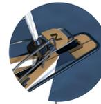
Easy removable stainless steel bow sprit for tacking of sails, anchor support and fitting a bow ladder.
