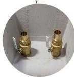
All through hull fittings are over dimensioned and fitted on single laminate. The reinforced hoses have twin clips in acid resistant stainless steel.
