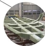
The hull is reinforced with a longitudinal and transverse floor grid system including stringers which also supports the keel fittings, bulk heads, keel stepped mast, engine frame, tanks, and cabin soles. The grid system is in the same material and E-module as the hull. Made in sandwich construction with vinylester on both inner and outer skin and Divynycell as core. It is glued and laminated to the hull. The whole structure is super strong and weighs about 900 kg.
