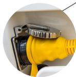
230V shore power system mounted in stern for easy access. Fitted with stainless steel intake, 25 m cable, fuse box, earth fault interruptor and four sockets.
