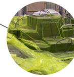
Vacuum infused hull and deck in sandwich construction including multi-axial fabrics, vinylester on both inner and outer skin and divynycell as core material.
