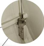
Stainless steel chain plates, bolted and laminated on both sides to the hull and grid structure.
